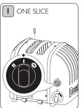
2 & 4 slot models: Rotate the 'selector switch' clockwise to the one slice indicator. The left hand slot will heat up on both sides.
